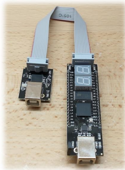
Figure 3: JTAG Cable Orientation
